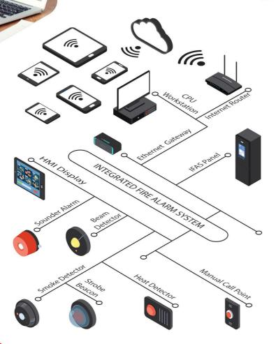
The novelty of system is real-time monitoring with many technologies combination to identify catastrophic event, historian and early notification ability via cloud computing
